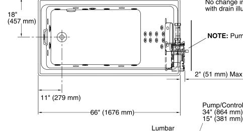
with drain illustrated. (K-7148-AF) **NOTE:** Pump/piping protrudes beyond rim.
